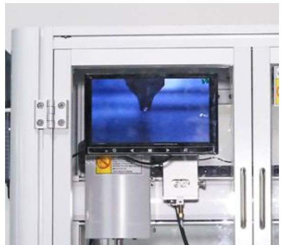
Vision options to monitor the soldering effect throughout the process, and can handle high-precision product soldering.
