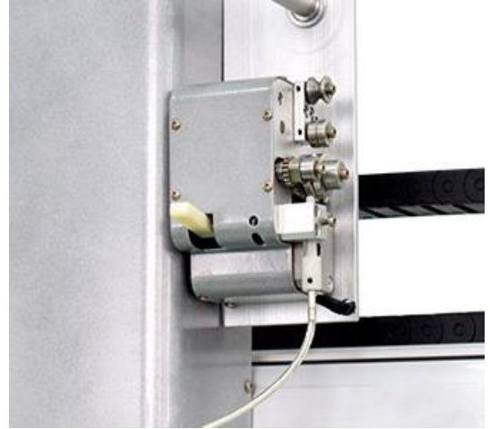
Special structural design ensures good supply of tin wire, no broken wire, stuck and other problems.
