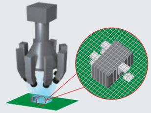
YRi-V performs high-speed height measurements within an entire field of view, in one batch. This 3D imaging reliably detects floating components that a 2D inspection can miss. Detection is also improved where color tones between board and components are similar or when there is interference between silk-screen and pattern. YRi-V 3D inspection can also detect the slope gradient and direction, and make pass/fail contour judgements.
