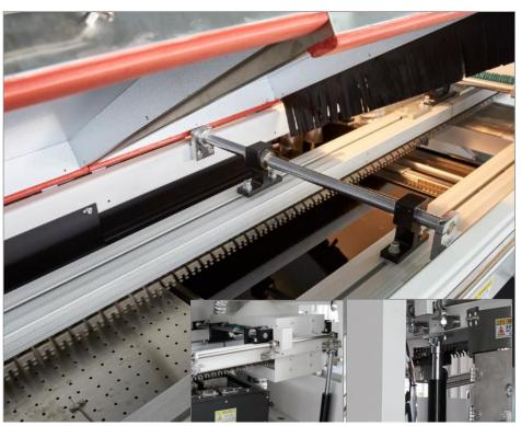
Heat-resistant and high-density aluminium support, no deformation.
