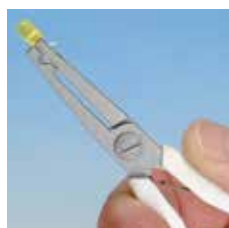
341A cut and form pliers put stress relief in component lead and trims to length with one squeeze.
