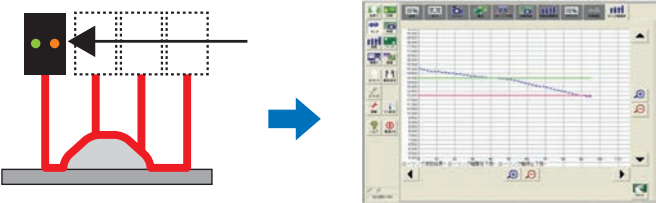
Measures rolling width of solder
